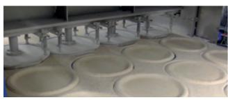
Various product shapes can be cut by the same cutting module and cutting change-over tools.
