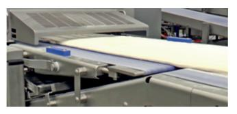
Elimination of falling heights: by minimizing the transportation height throughout the production line, it results in a stable and relax dough sheet.
