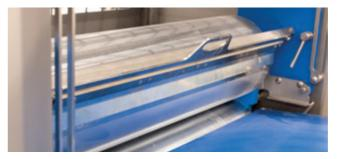
Wear resistant roller scrapers are used to keep the rollers of the reduction stations as clean as possible.
